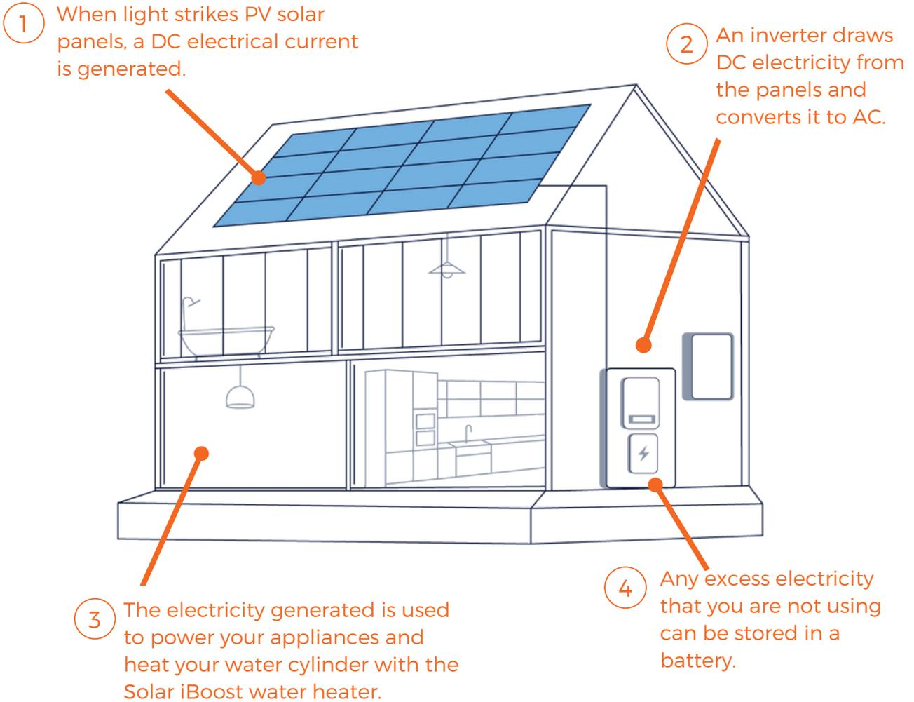
Each panel is 1 metre in width, and 1.8 metres in length. A 4kW system will generally require 10 panels.
